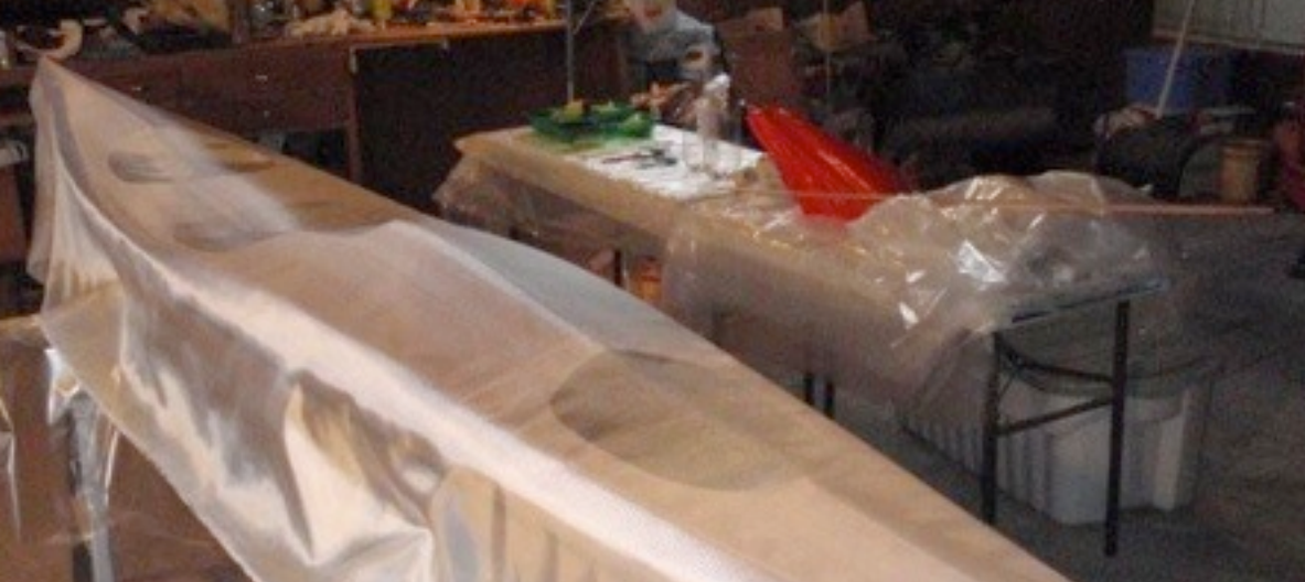
The hull with the deck joined to it, and the fiber-glass cloth is draped over the deck ready to fiberglass.
