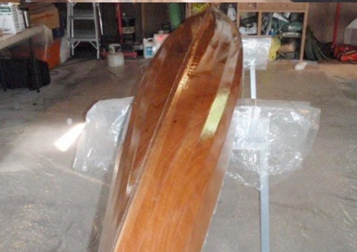
The Hull with fiberglass coating applied
